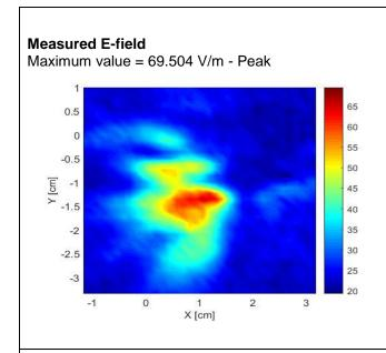
Reconstructed localized free space power density Maximum value = 0.582 mW/cm<sup>2</sup>
