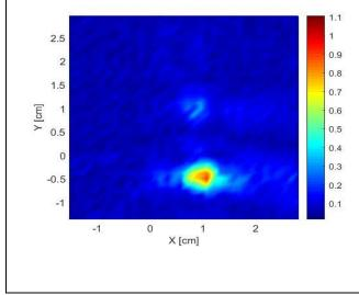
**Reconstructed H-field (from Measured E-field)** Maximum value = 0.221 A/m - Peak
