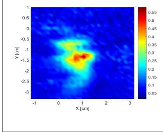
**Reconstructed H-field (from Measured E-field)** Maximum value = 0.227 A/m - Peak
