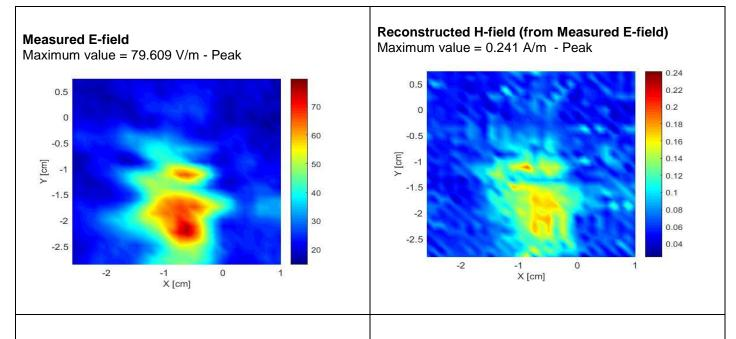
Reconstructed localized free space power density Maximum value = 0.697 mW/cm<sup>2</sup>
