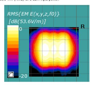
The plots below show the comparison between the calibration certificate and the system check results in terms of normalized E-field distribution and the 1D variation along the two axis of the maximum.
