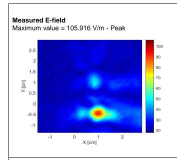
Reconstructed localized free space power density Maximum value = 1.105 mW/cm<sup>2</sup>
