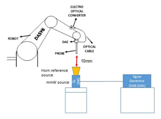
The output power on the reference source is set to 5.0 dBm (3.16 mW) and E-field results are normalized to a forward power of 10mW to compare the values with the calibration report.
