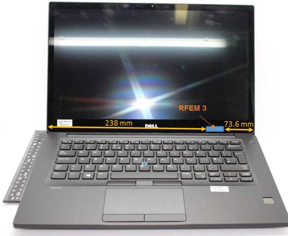
Figure 18 – Platform picture with RFEM 3 location
