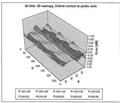
Probe isotropy for E<sub>tot</sub>: probe rotated  $\phi$  = 0° to 360°, tilted from field propagation direction  $\overline{k}$  Parallel to the field propagation ( $\psi$  =0° - 90°): deviation within ± 0.38 dB Normal to field orientation (9 =0° - 90°): deviation within ± 0.47 dB
