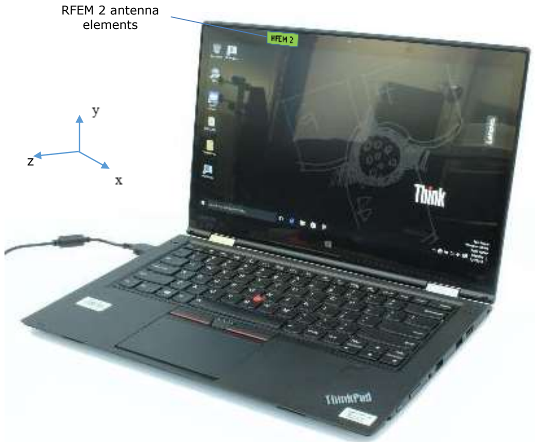
Figure 7 – Active antenna inside the platform
