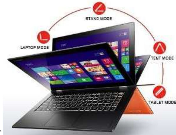
Figure 5 - Platform operating modes
