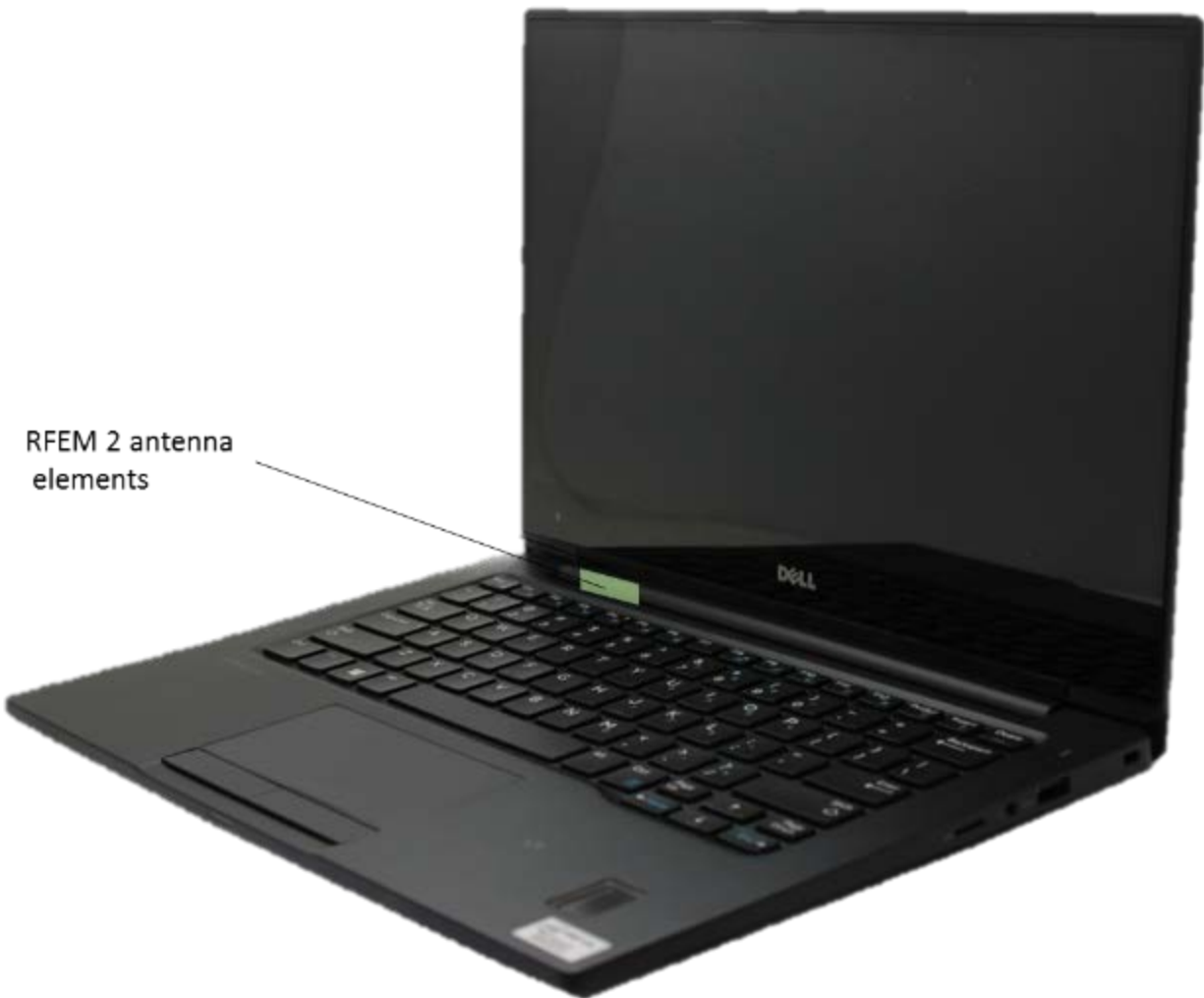
Figure 6 – Active antenna inside the platform
