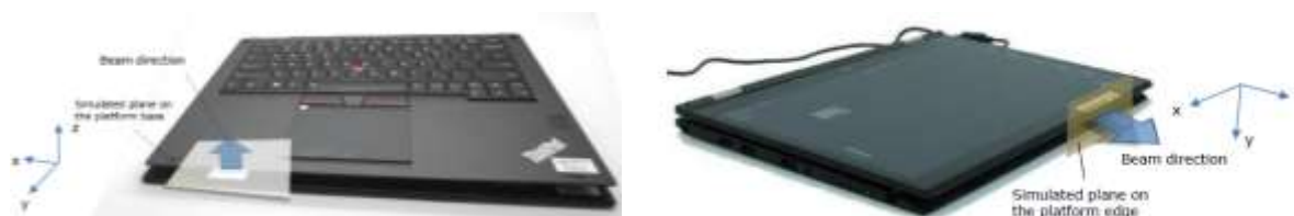
Figure 3 – Search Planes are the x-y planes (i.e. the transparent plane as illustrated in this picture- Left: Base plane Right: Edge plane)
