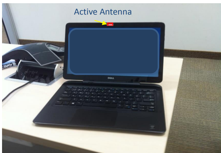
Figure 7– Active antenna inside the platform
