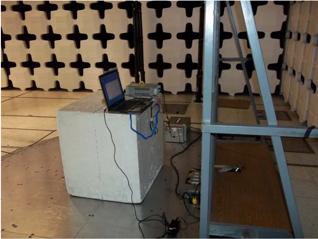
Conducted Emissions Test Configuration Photograph
