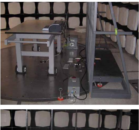
AC Power Line Conducted Emissions Test Configuration Photographs
