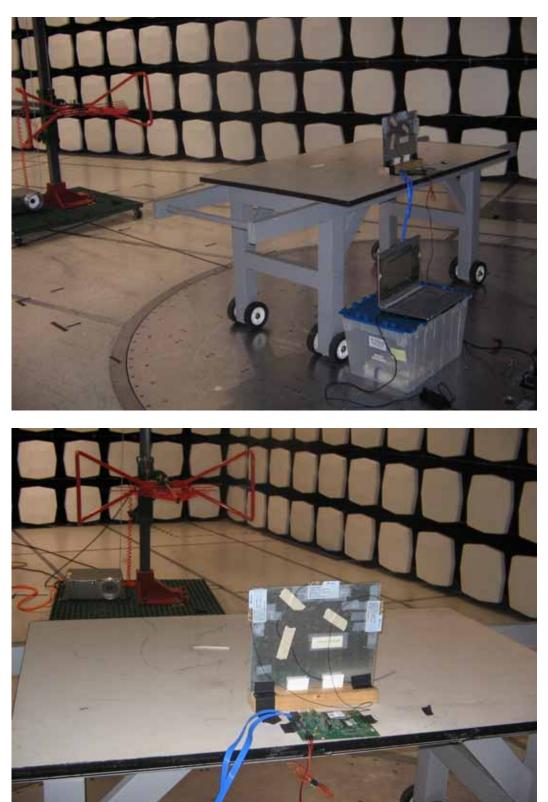
Radiated Emissions Test Configuration Photographs
