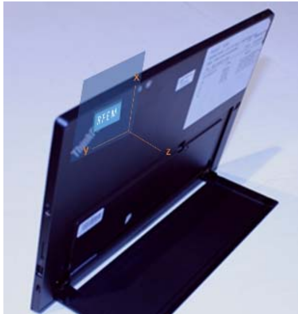
Search Plane is the x-y plane (i.e. the transparent plane as illustrated in this picture)
