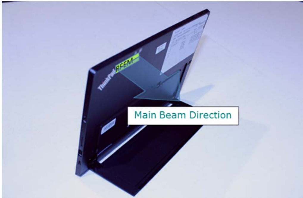
Figure 3– Active antenna inside the platform
