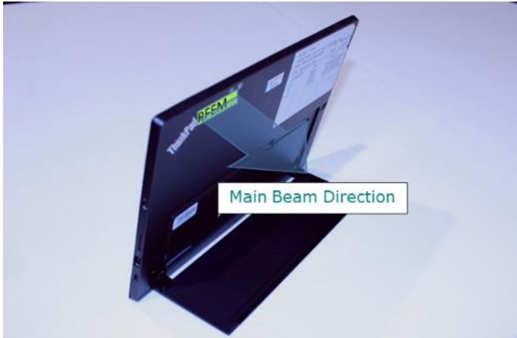
Figure 3– Active antenna inside the platform
