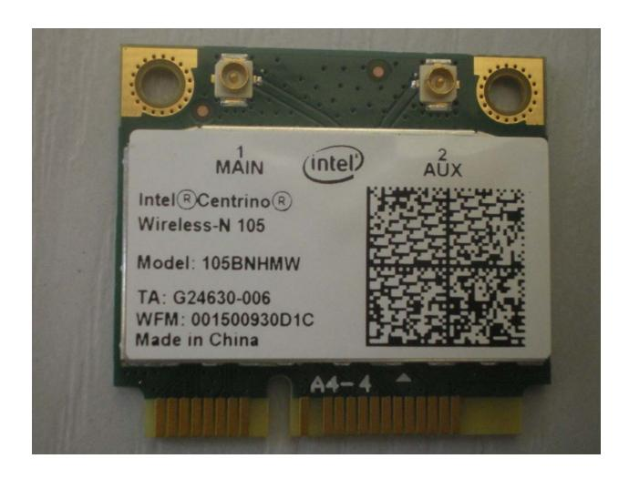
Photos shows label placement on half-mini card Label wraps around onto the other side of the board. The side of the label with the FCC ID appears on the back of the board.
