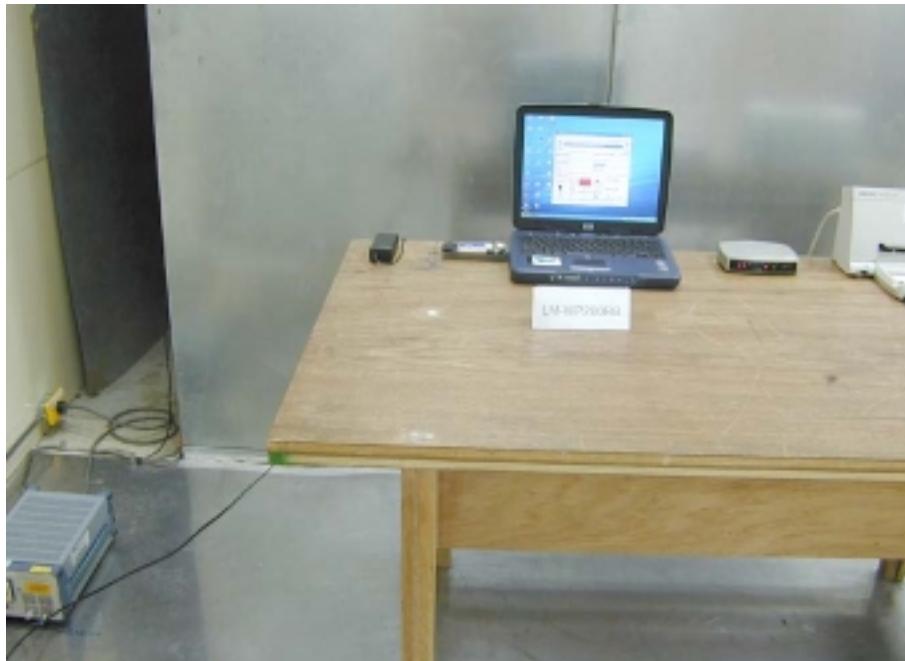
Appendix C2: Conducted Emission Test Set-up (rear)
