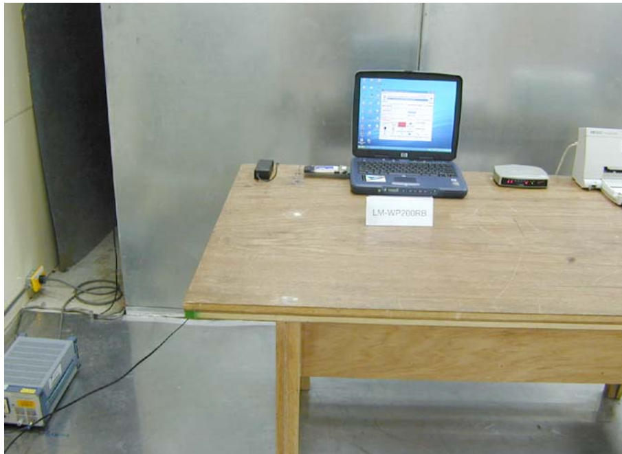
Appendix C2: Conducted Emission Test Set-up (rear)
