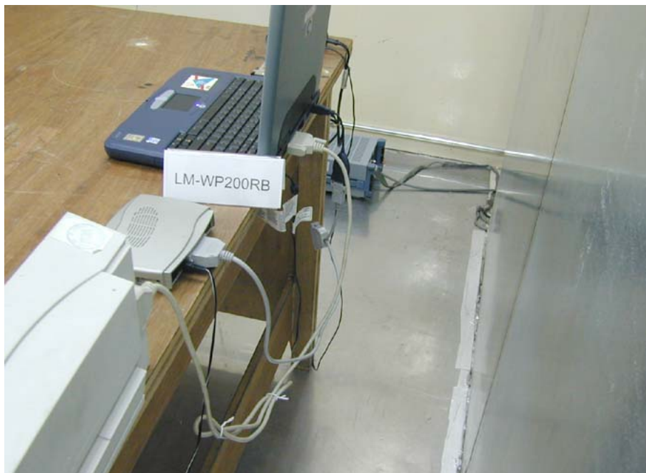
Appendix C2: Conducted Emission Test Set-up (rear)
