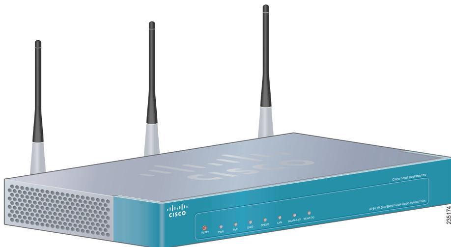
**PWR**—Lights green while the access point is powered on. Blinks during a firmware upgrade.
