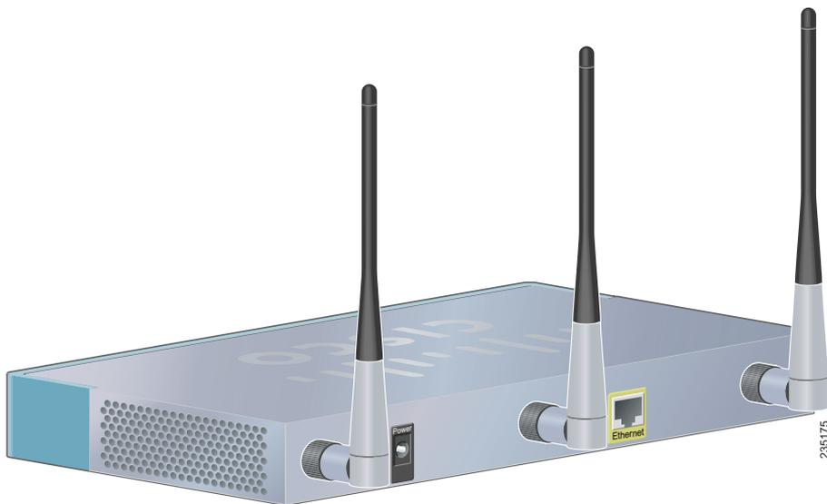
**Ethernet Port**—The access point is equipped with an auto-sensing, Gigabit Ethernet (802.3) port used for configuration and wired network communications. Auto-sensing technology enables the port to automatically detect the speed and duplex settings of the device connected to it, and adjust its speed and duplex settings to match the settings of the connected device. The Gigabit Ethernet port accepts an RJ-45 connector and supports Power-over-Ethernet (PoE).
