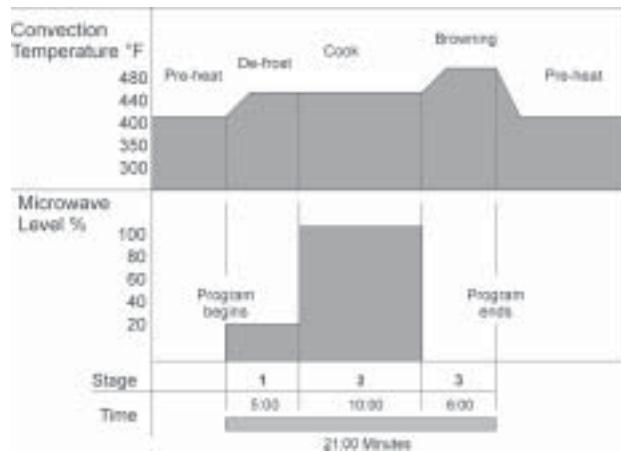
A typical 3-stage program is shown. The Oven is pre-heated at 350°F. Stage 1 begins by applying a gentle microwave power of 25% (ideal for defrosting) while the convection temperature rises to 440°F. In Stage 2 the microwave power increases to maximum (100%) . In the final, browning stage the convection temperature is increased to 480°F with no microwave energy applied.
