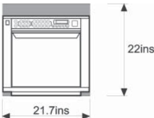
To meet NSF requirements the oven needs to be sealed to the worktop to prevent ingress under the oven
