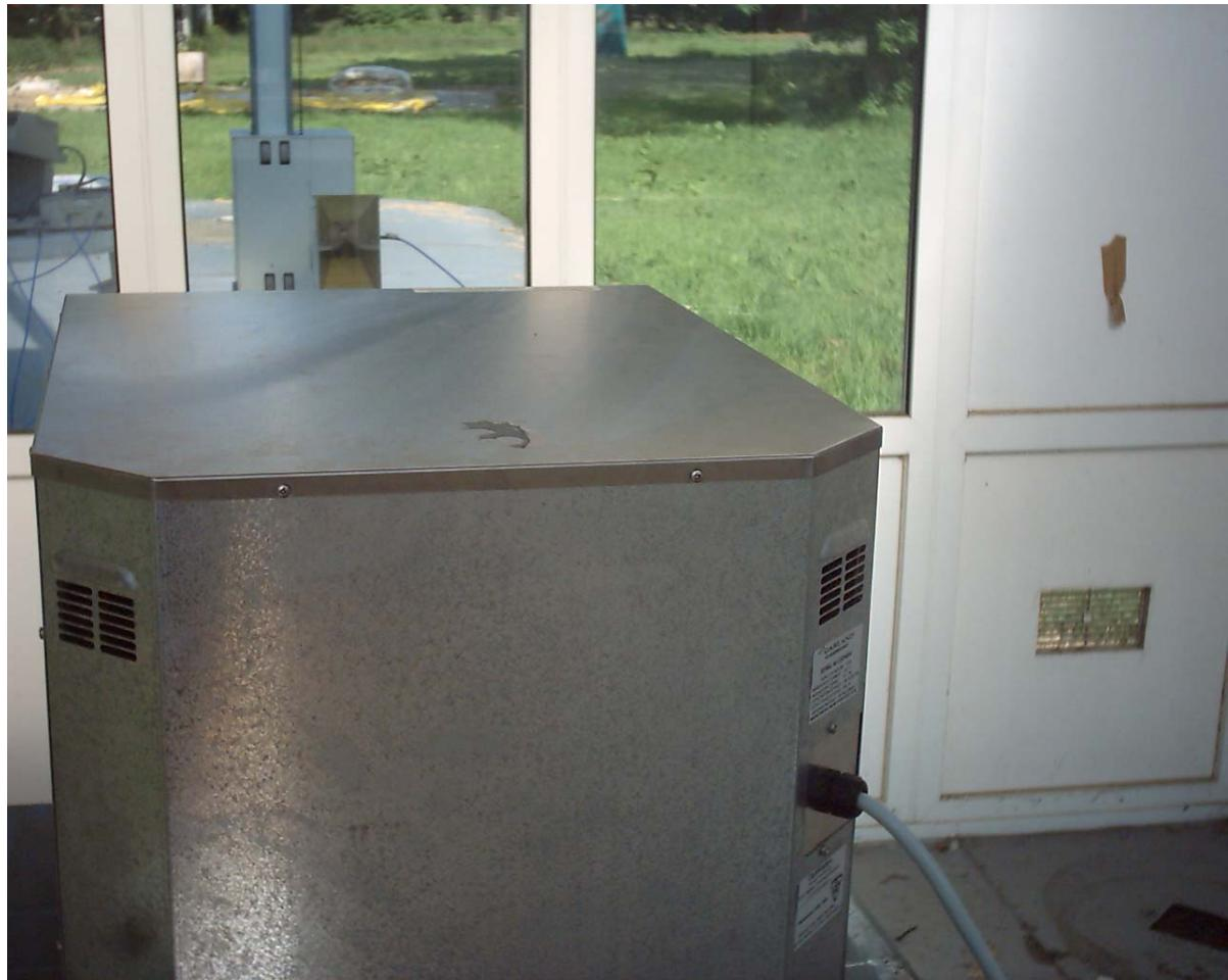
8.1.4.1 Test 1b - Figure 2 – 208 V Oven – 2.4 GHz-2.5 GHz OATS
