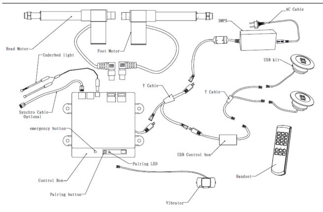
The control box is designed for using the SMPS of 29VDC/ around 2A as the power. It is necessary to use the SMPS provided by us when normal operation.
