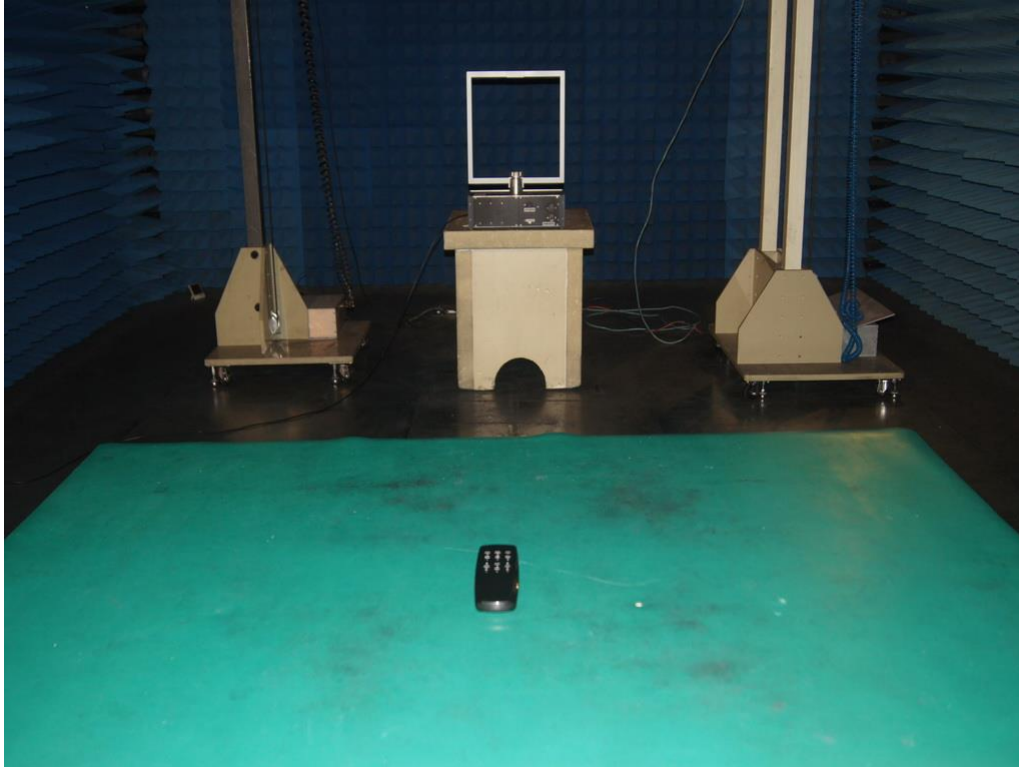
Photograph 2: Set-up for Spurious Emissions of 30MHz – 1GHz
