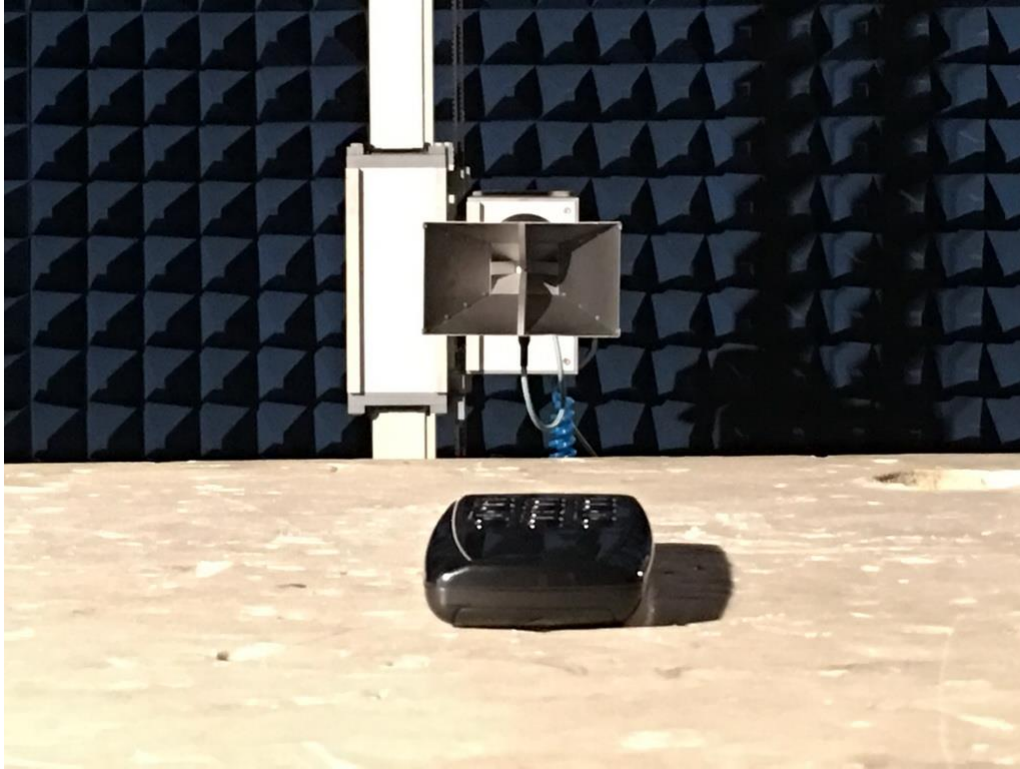
Photograph 4: Set-up for Spurious Emissions of 18 – 26.5GHz
