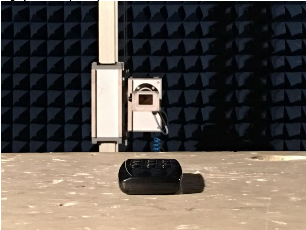
Photograph 4: Set-up for Spurious Emissions of 18 – 26.5GHz
