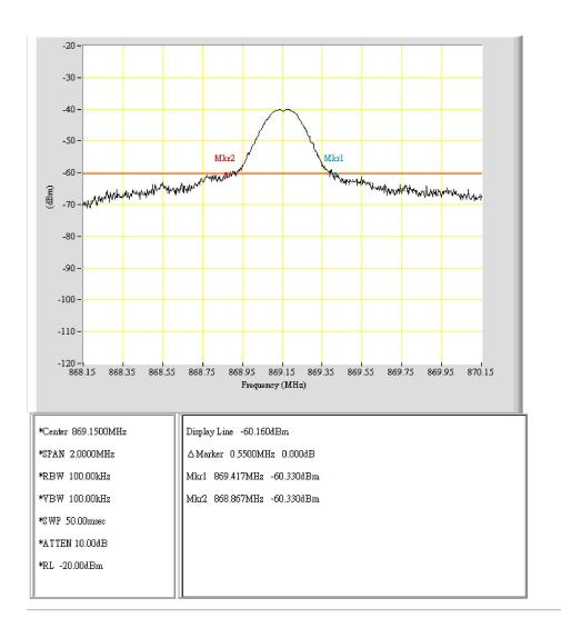
EUT: A5-PROP Purpose: 20dB\_BW Condition: Tx\_868\_CH20
