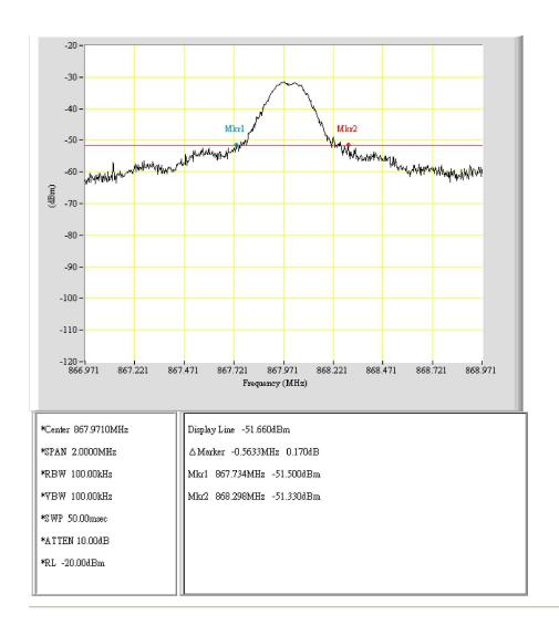
EUT: A5-PROP Purpose: 20dB\_BW Condition: Tx\_868\_CH1
