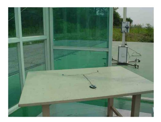
■ Radiated Test Picture (Playing mode & FM broadcast receiver mode -Rear)
