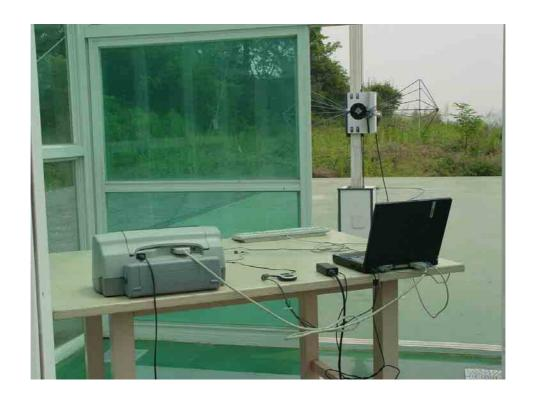
■ Radiated Test Picture (Playing mode & FM broadcast receiver mode - Front)
