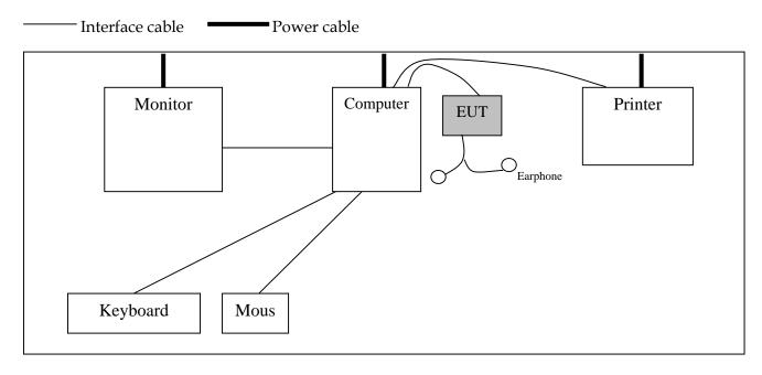
**5.4 Peripherals / Support Equipment Used**Following peripheral devices and interface cables were connected during the measurement:
