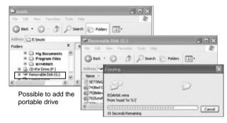
If USB drive connects to the computer, the message such 'USB Connected...'show up.The message such 'USB Connected...'and LED flicker During the transfer, otherwise they didn't flicker and then USB drive separate from the computer.
