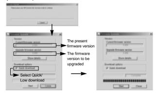
Note: In the case of the progress bar's not being proceeded in the above figure, it shows that the USB drive is not connected normally. In this case, push the play/stop button after disconnecting an USB drive with PC and reconnection the USB drive to the PC.
