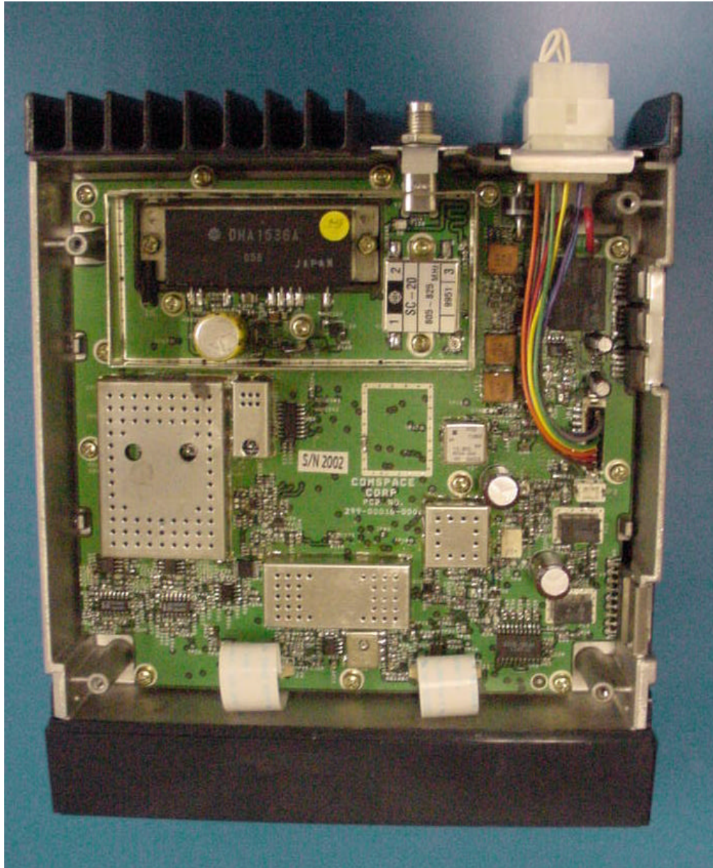
Top cover removed showing RF PCB
