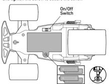
Slide battery cover off. Insert the 9V battery matching the polarity etched in the battery tray. Replace battery
