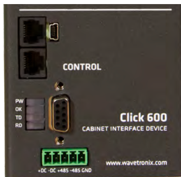
Figure D.4 - Control Bus
