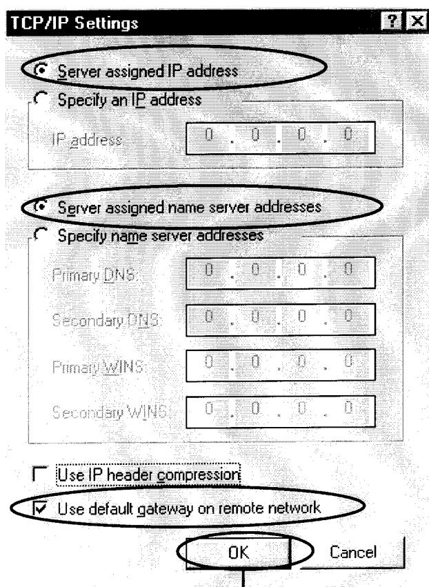
⑫ Select 'Server assigned IP address', 'Server assigned name server addresses' and 'Use default gateway on remote network'. Then click 'OK' two times.
