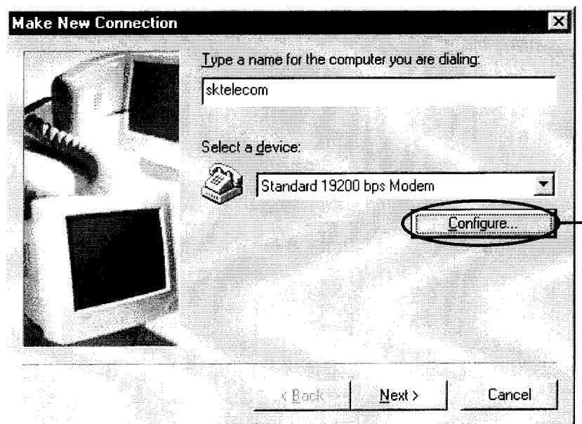
② Type the service company name to be used at 'Type a name for the computer you are dialing' and select 'Standard 19200 bps Modem' for 'Select a device', then click [Configure].
