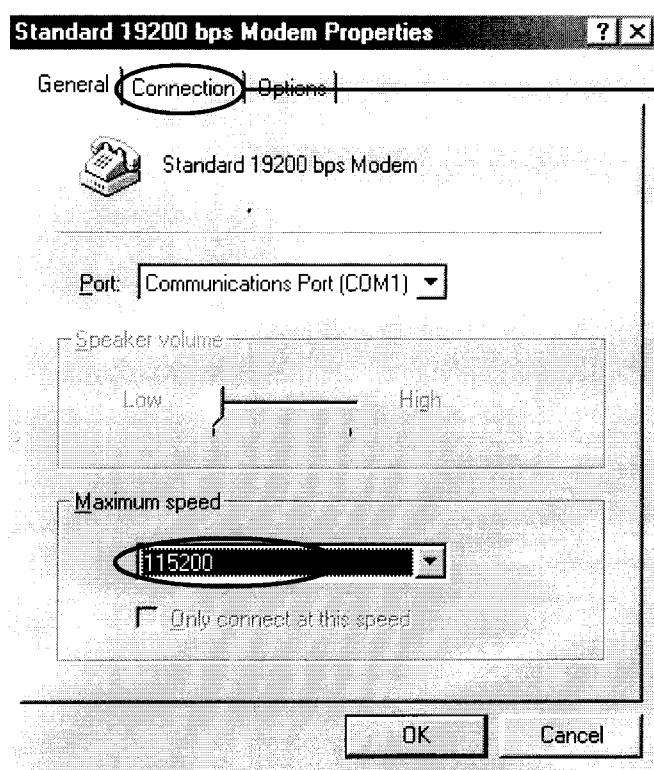
③ After confirming 'Communication Port (COM1)', select '115200' for 'Maximum speed(bps)', then go to 'Connection' folder.
