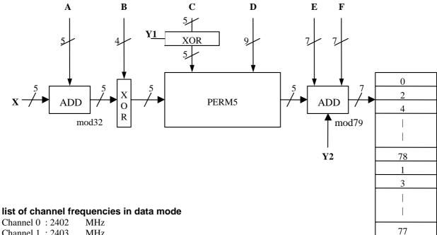
Channel 0: 2402 Channel 1: 2403 MHz Channel n : 2402 + n Mhz Channel 78: 2480 MHz
