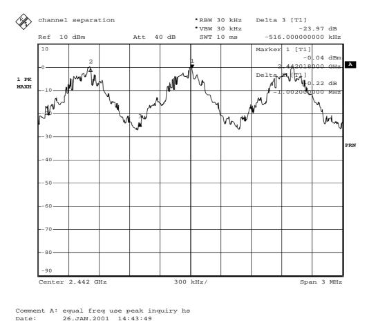
This is evidence the device has hopping channel carrier frequencies separated by 20 dB bandwidth of the hopping channel.
