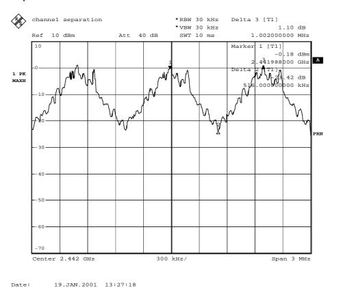
This is evidence the device has hopping channel carrier frequencies separated by 20 dB bandwidth of the hopping channel.
