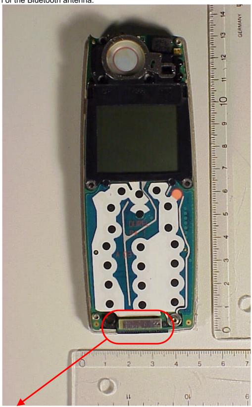
The Antenna is placed on the front side over the system connector (small long grey thing within the red circle). The antenna is a non-uniform omni directional PLIFA (Planar Inverted F Antenna)
