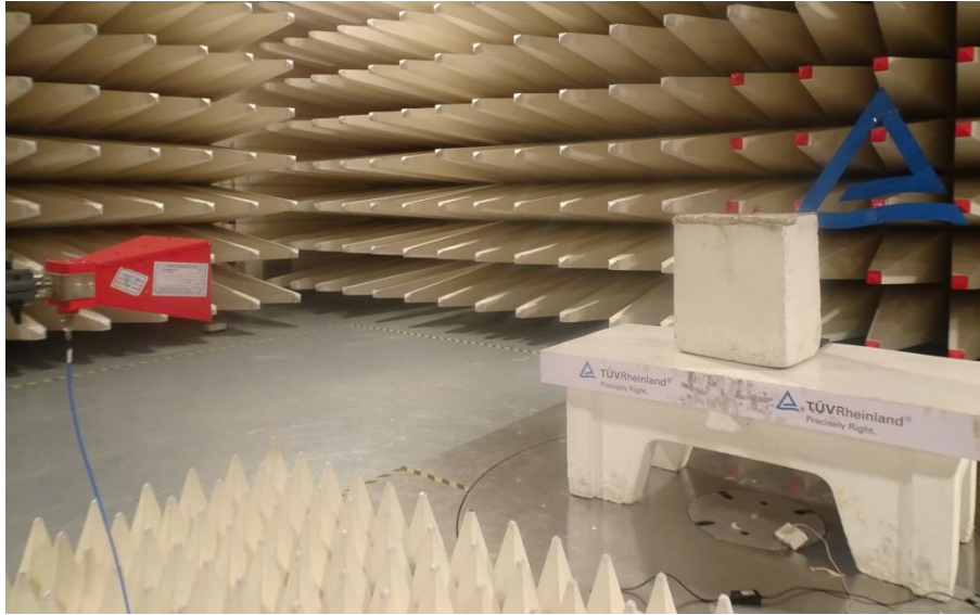
Photo 7: Horn antenna with vertical polarization
