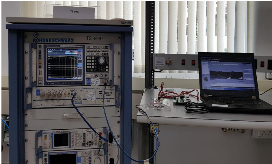
Photo 13: Antenna port measurement setup
