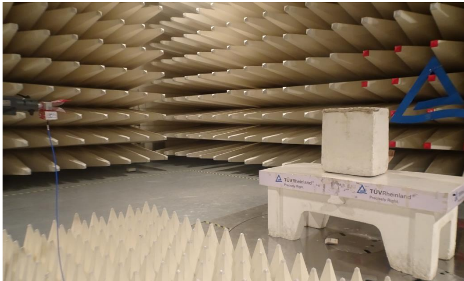
Photo 9: Horn antenna with vertical polarization
