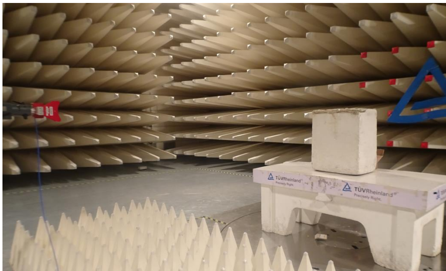
Photo 10: Horn antenna with horizontal polarization
