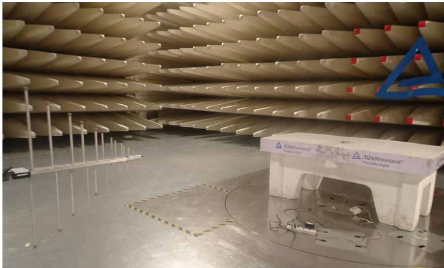
Photo 5: Log periodic antenna Vertical polarization
