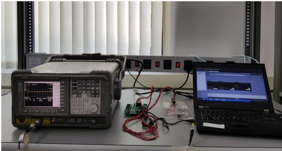
Photo 14: Antenna port measurement setup
