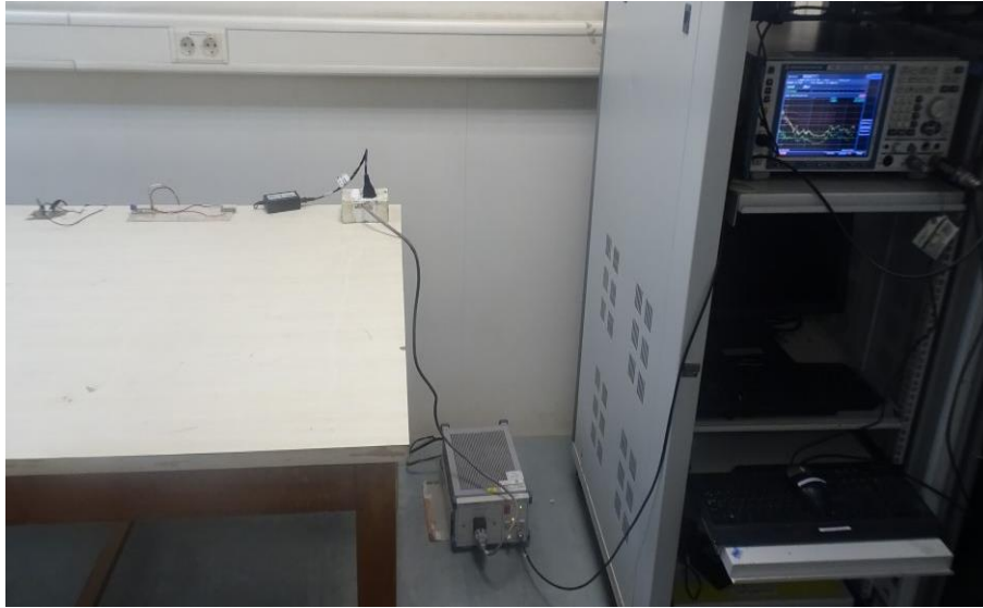
Photo 15: Conducted Emission Setup
