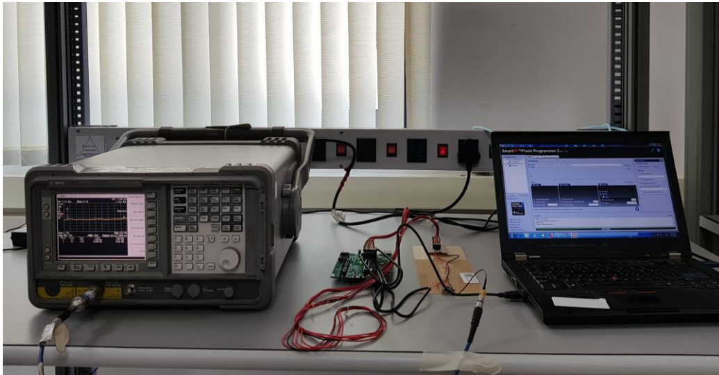
Photo 13: Antenna Port measurement
