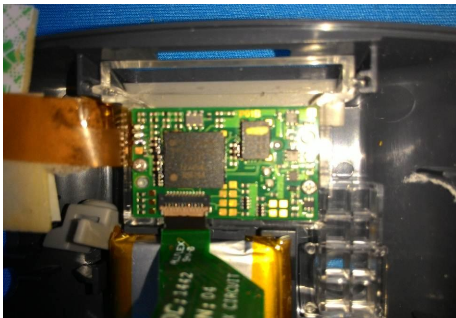
EUT Barcode Reader Circuitry
