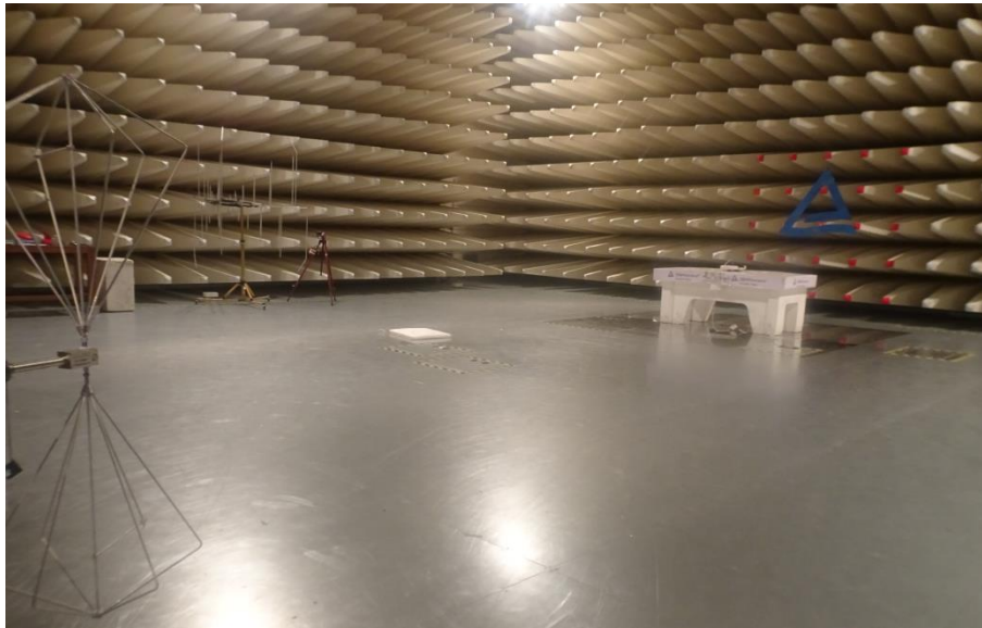
Photo 3: Biconical antenna vertical polarization
