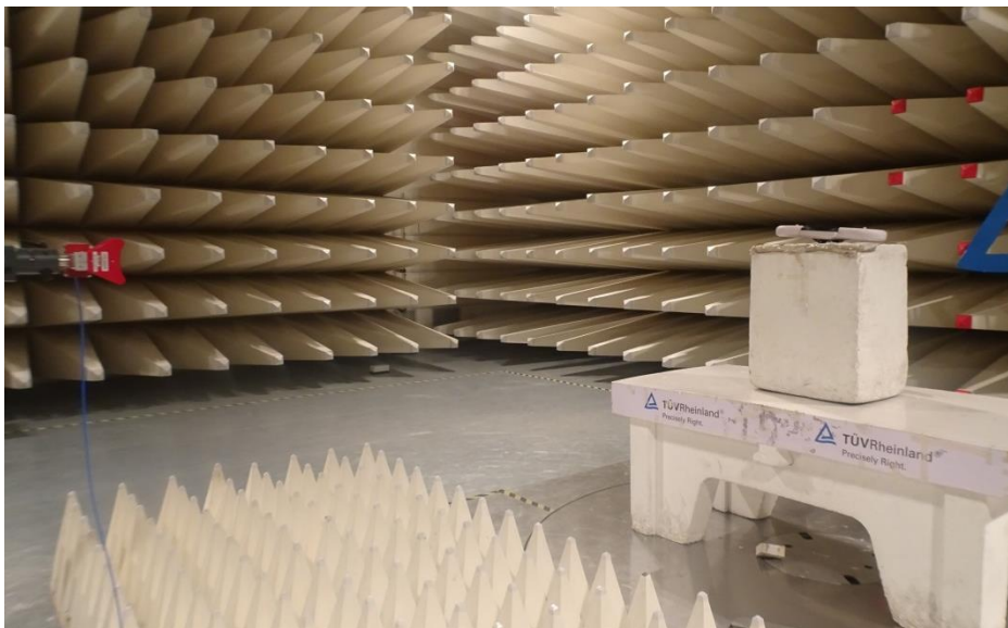
Photo 10: Horn antenna with horizontal polarization
