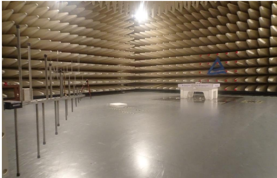
Photo 5: Log periodic antenna Vertical polarization
