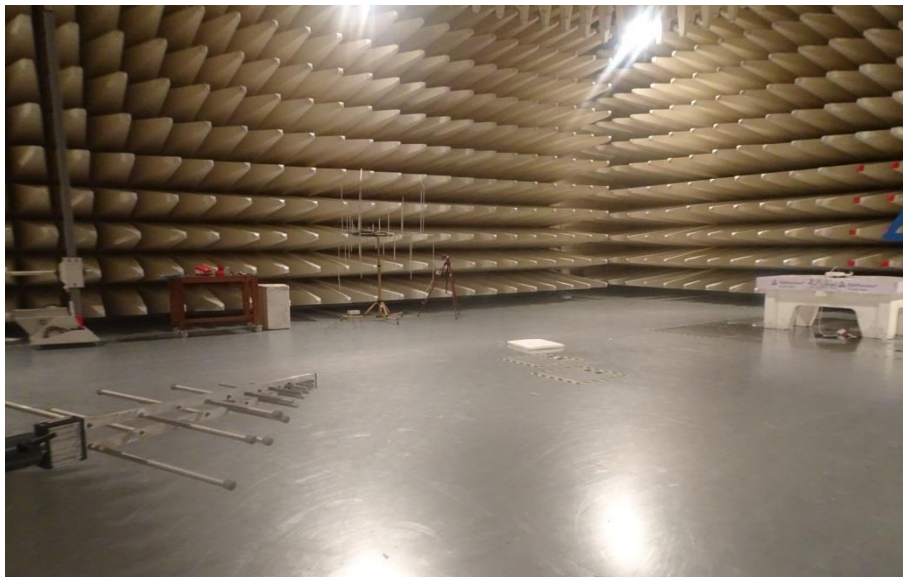
Photo 6: Log Periodic antenna Horizontal polarization
