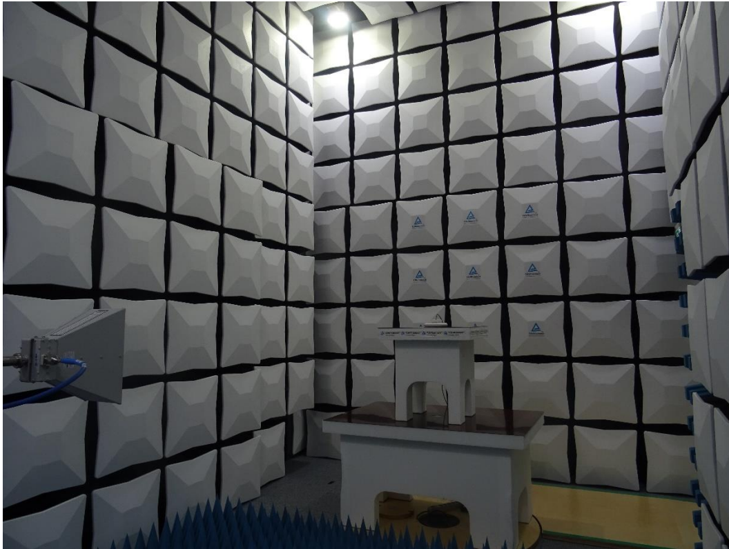
Photo 9: 1GHz to 18GHz - Horizontal polarization
