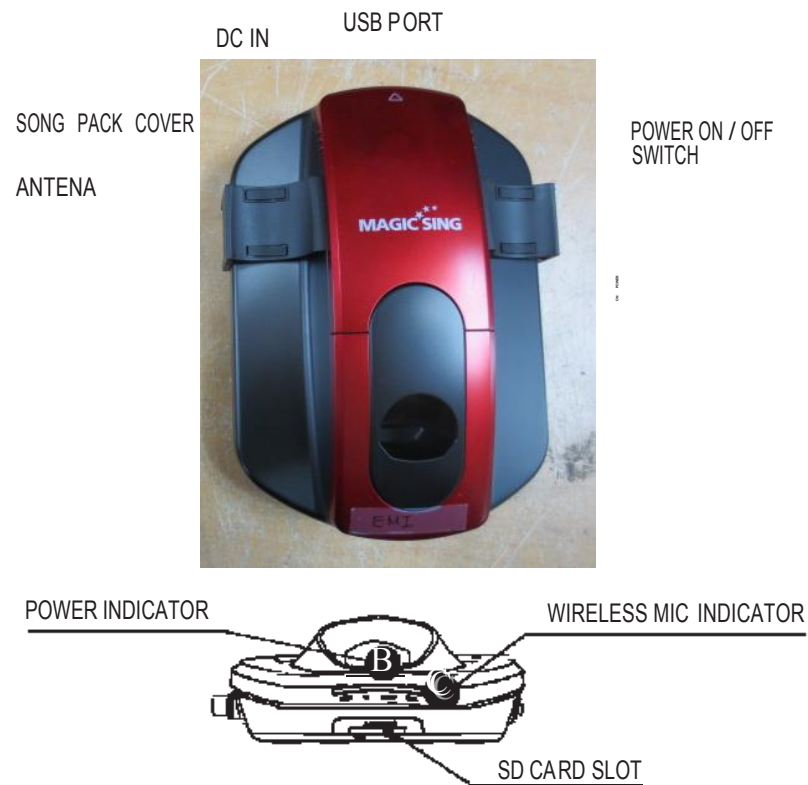
ET23KM Main Station
