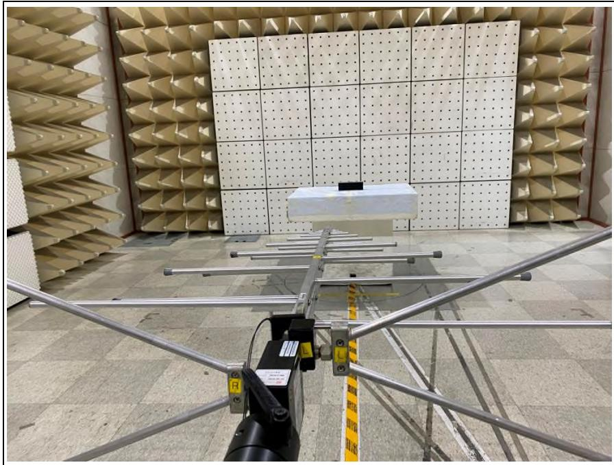
**3. Photo of Radiated Spurious Emission Test (Above 1 GHz)**
