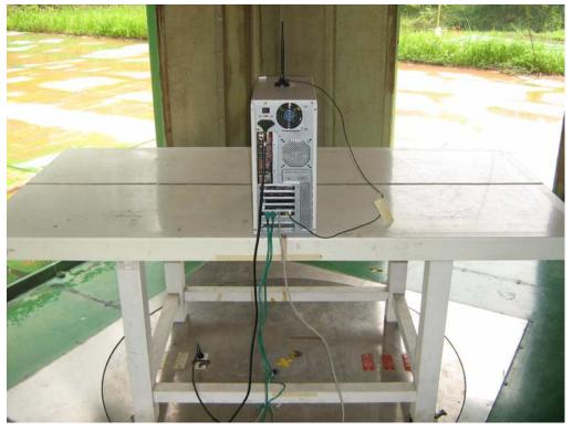
RADIATED RF MEASUREMENT SETUP
