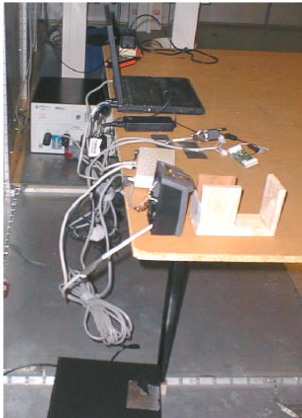
**Test set-up, Conducted Emission**
