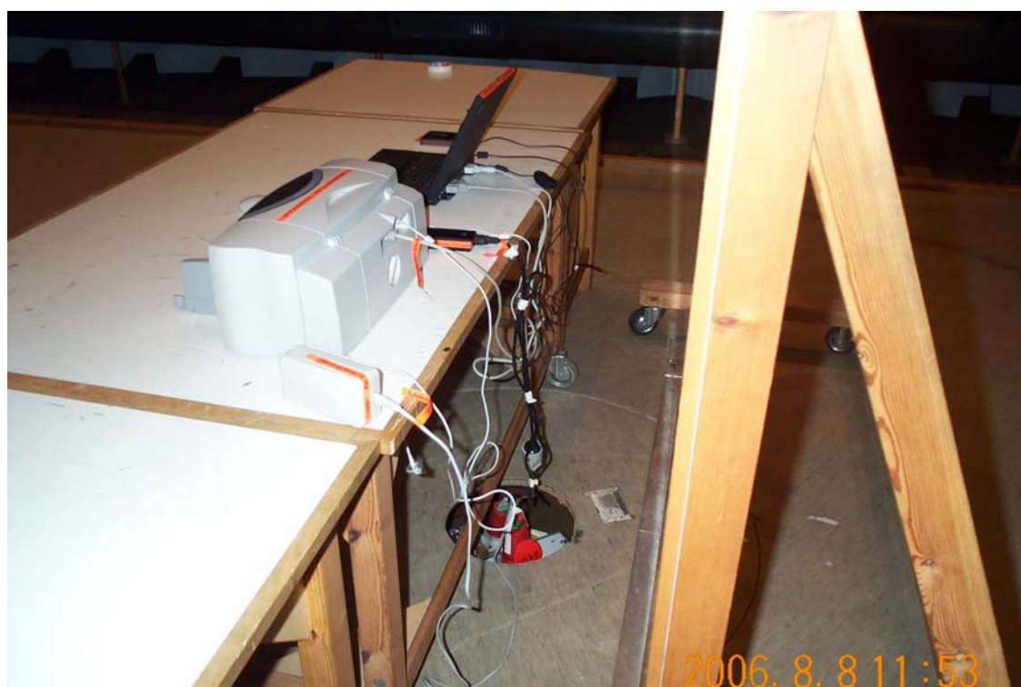
Photo 4.1.2 Test setup regarding measurement of RF voltage on AC mains.
