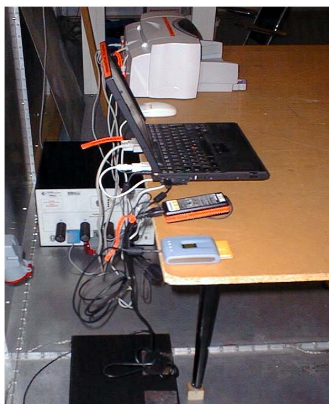
**Test set-up, Radiated Emission**
