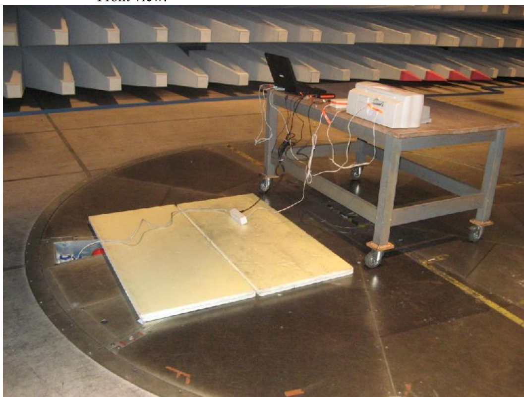
Photo 4.2.2 Test setup regarding measurement of radio frequency electromagnetic field. Side view.
