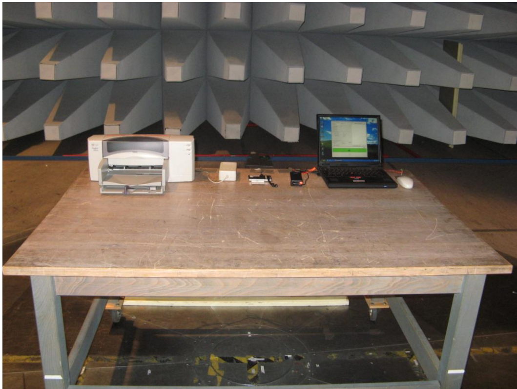
Photo 4.2.1 Test setup regarding measurement of radio frequency electromagnetic field. Front view.
