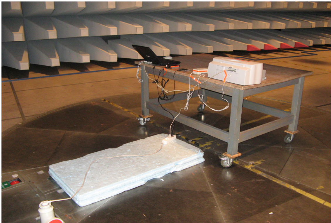
Photo 4.2.2 Test setup regarding measurement of radio frequency electromagnetic field. Side view.
