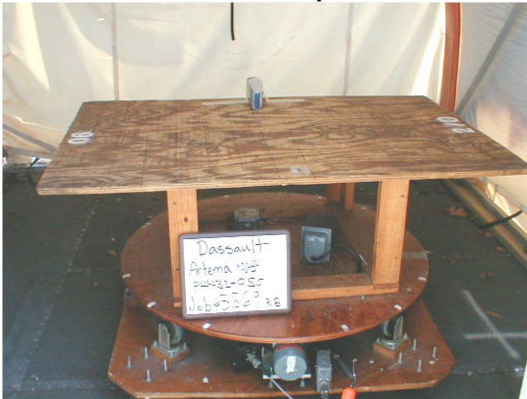
Radiated Emissions Test Setup – Back View
