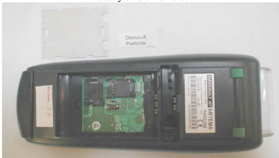
Battery Shield Removed
