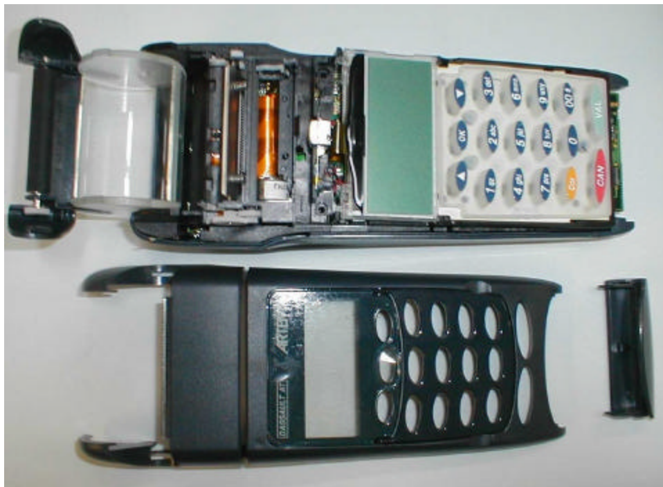
Front Cover Removed
