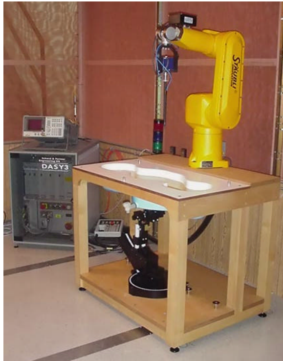
Figure 5. DASY3 SAR Measurement System
