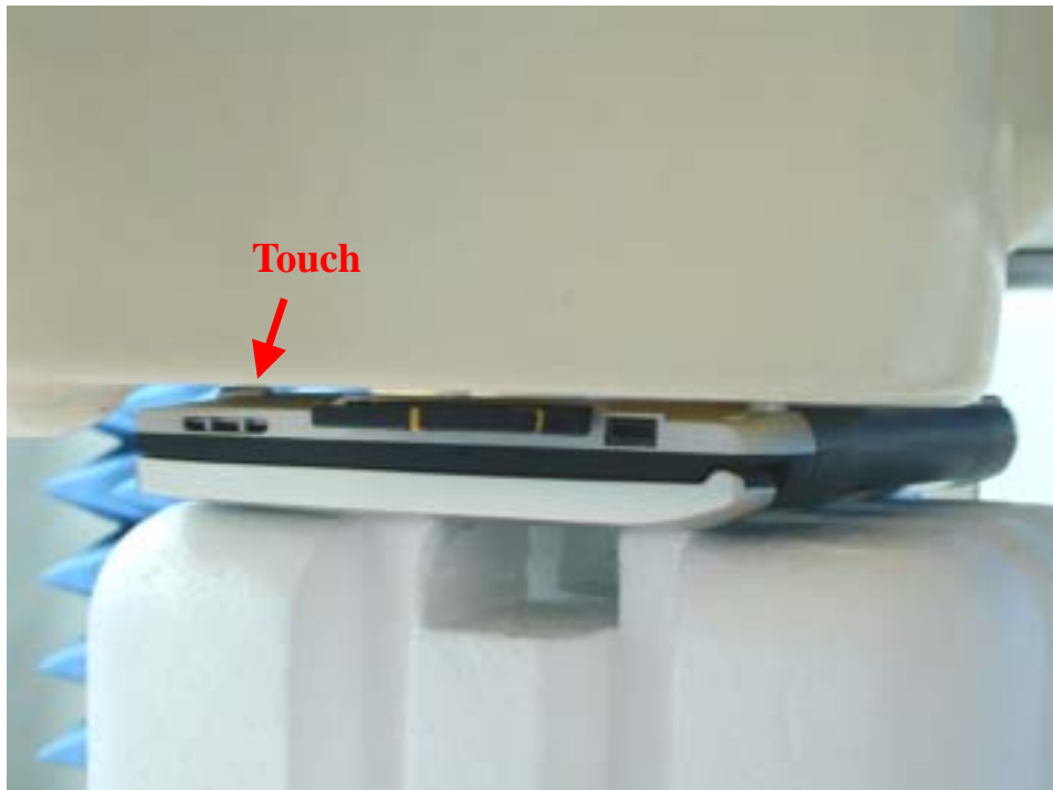
Fig.6 Photograph of the Bottom of the Pc is paralleled and at a distance of 0.0 cm from the base of the phantom, but 0.5 cm Spacing between EUT & Planar Phantom.
